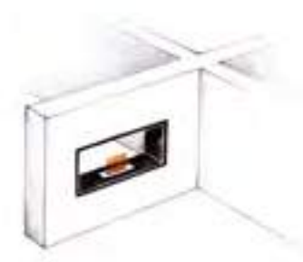
Foyer traversant (1) Through-wall fireplace (1)
